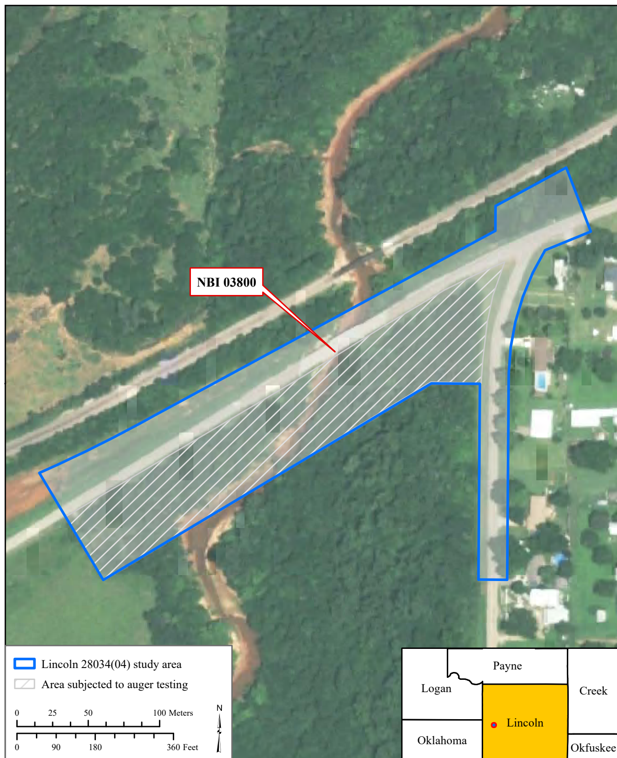
Figure 2. Lincoln 28034(04) SH-66B bridge over Captain Creek, 1.5 miles northeast of SH-66; showing areas subjected to auger testing.
