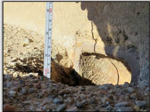
Figure 8. Measuring Asphalt Overlay Depth at Deck Drain Location
